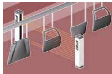
Detection of position and profile of workpieces in automated painting systems
